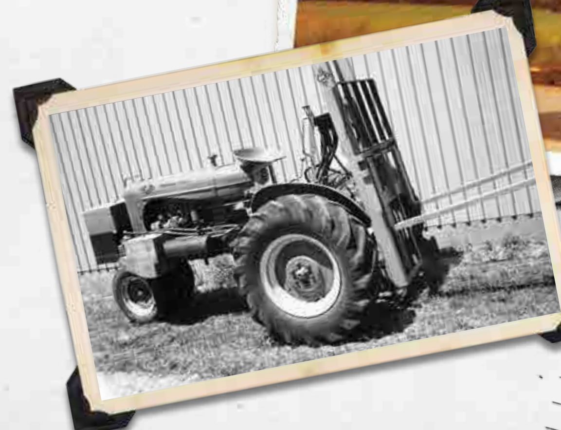
An Allis Chalmers tractor that was retrofitted with a forklift mast designed by G. White Industries.
